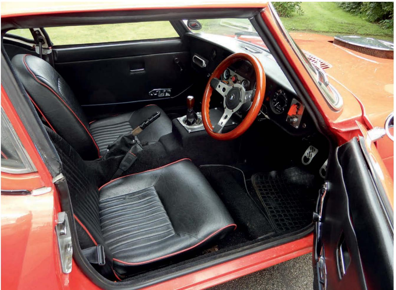
The interior remains mostly standard, although the transmission tunnel is now made of steel rather than cardboard, and has become a structural member.
