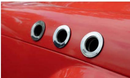
Buick-style portholes will be quite good at providing an outlet for hot engine bay air.
