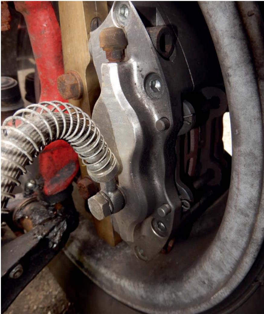
Wilwood performance brake calipers add some bite to the brakes. Tripling the engine power does require some concomitant upgrades.
