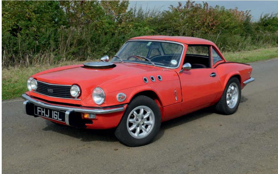
Looking at the car more from a three-quarter angle, the changes to the bonnet continue quite far back along its length. A pair of SU carbs on a copy of an MGB V8 inlet manifold or copy thereof could probably have been hidden under the bonnet.
