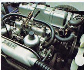
The Spitfire's distinguished 1493 cc engine is incredibly strict with its fuel—but enormously generous with its power. Developing 71 b.h.p. at 5,500 r.p.m. the sharp, confident acceleration can take you up to the 100 mph mark. And steady cruising at 50 mph can give you real economy, enhanced further by the optional overdrive—up to 50.6 miles to the gallon.\*
