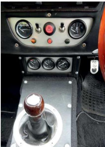
Instrumentation is now rather more comprehensive, and includes an oil temperature gauge as well as coolant temp.
